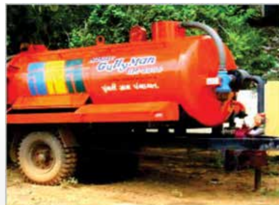
Tractor trailer to cleanup sewage Punsari Village, Gujrat
